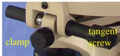
There are three clamp and tangent screw pairs: two (upper and lower) for horizontal circle adjustments, and one for vertical. In each case, the clamp is loosened to move the transit more than a few degrees, then the clamp is tightened for fine adjustment with the tangent screw
